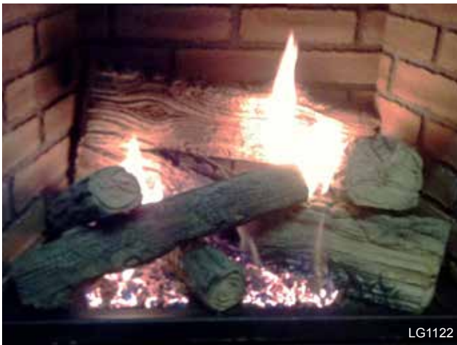
Figure 51 - Typical Burner Flame
